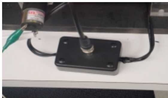
Illustration 11. Solid State Relay.
