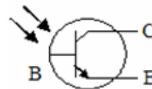
Figure 6: Schematic of phototransistor
