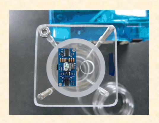
One final touch we needed was to provide a cover for the installation of our mechatronic components that allows us to automate the process of data collection in a falling head permeability test.
