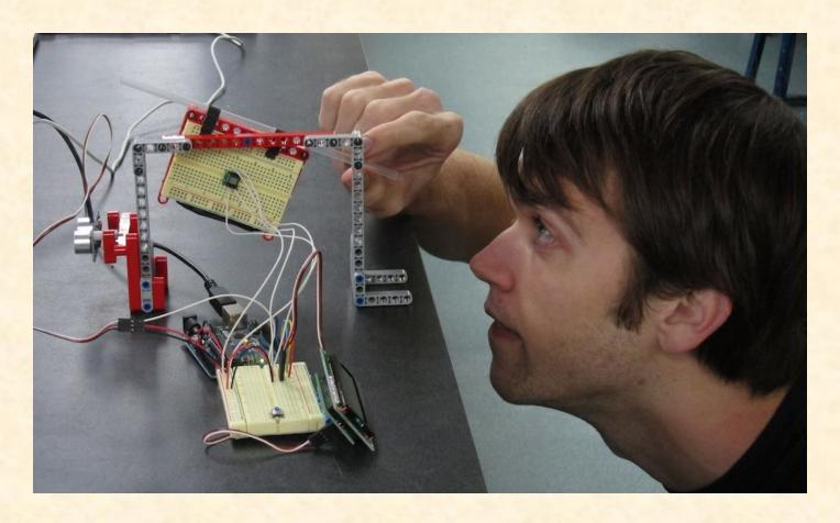
We relocated the pivot point so the center of the straw was right on top of it.
