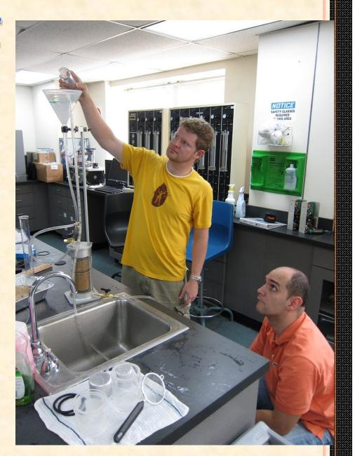
Our first test was to run a permeability test on a sand mixture. We used the ELE permeameter to determine how fast water could flow through the sample. This device was cumbersome, messy, and expensive.
