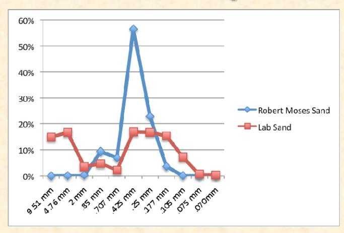
Neither of the sand samples were well graded, where particle size would be evenly distributed. A well graded soil will have less void space, lower permeability, and greater structural integrity.
