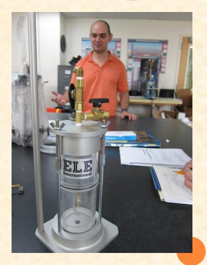
We set out to redesign the permeameter in a way to make it neater, more affordable, and K-12 friendly. Water flow in soil has a direct connection to the NYC Science Scope and Sequence
