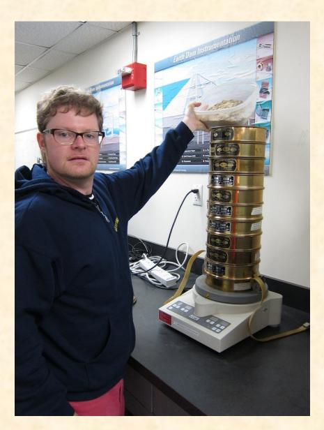
Next we poured the soil into the sieve stack. The openings get smaller and smaller each level down. The machine on the bottom shakes the stack to sort out the particles by size.
