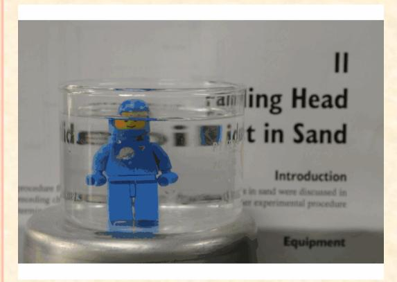
The Soil Mechanics Lab focuses their research on transparent soils. Transparent soils allow us to see what is happening inside the soil, This could be helpful to monitor what happens inside the soil when a force is applied or how a contaminant travels through soil. The LEGO man disappears over time because we added Aquabeads to the water. Aquabeads are a a water absorbing polymeric gel. They grow 200x their original size.
