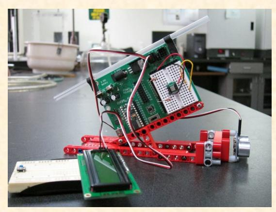
We decided to make a mechatronic clinometer. This was a first prototype, but the math was flawed. The height of the pivot point for the straw was not constant.
