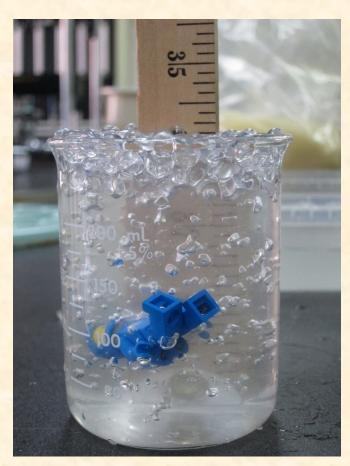
Transparent soils become transparent when we fill the void space with a liquid with a matching index of refraction. Aquabeads have the same index of refraction as water.
