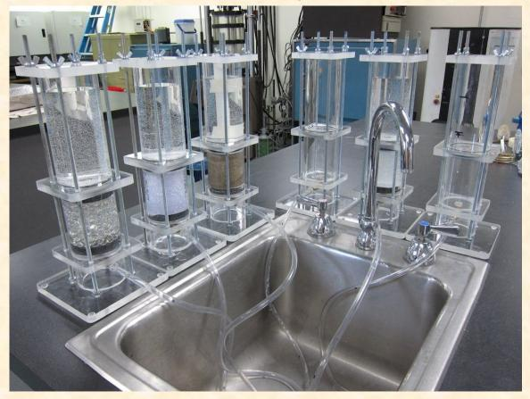
We built five more permeameters after being satisfied with the prototype. We now have two sets of three permeameters. This will allow us to run three concurrent tests in our respective classrooms.
