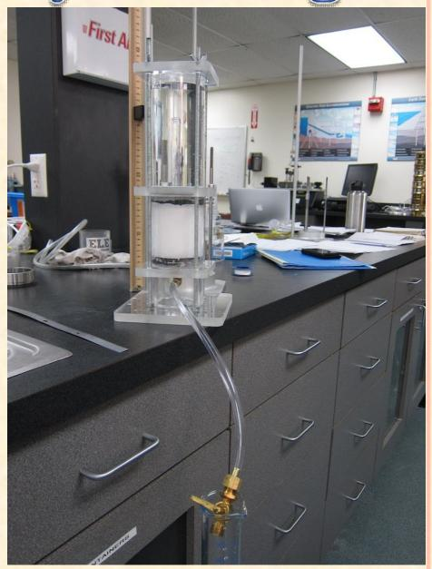
For each soil specimen, we recorded measurements to calculate the void ratio. Additionally, we conducted sieve analyses for two separate soil samples. Running the permeability test allowed us to measure the actual coefficient of permeability for each type of soil.
