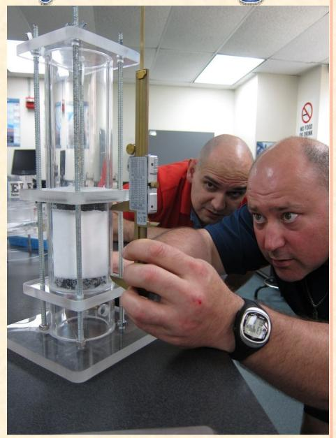
We began each test by measuring the mass and volume of the sample. We then timed the duration for the sample to pass 205mL of water. We also noted the difference between the starting head height and the ending head height.
