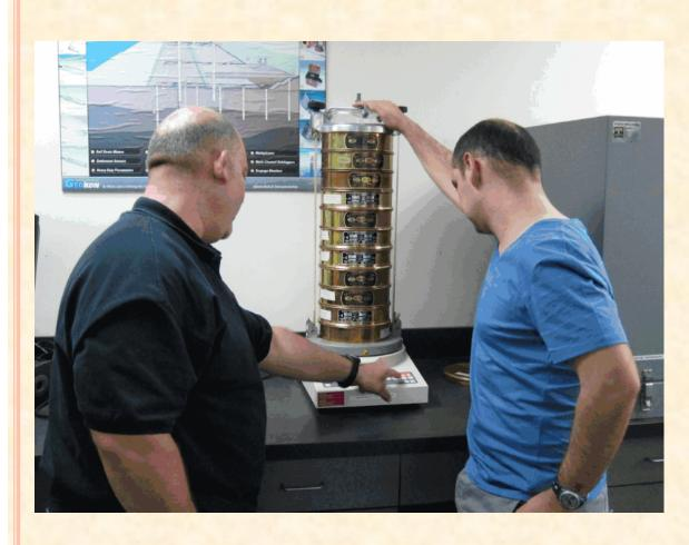
The sieve analysis allows us to quantify mass distribution by particles size. It does not distinguish between clay and silt. Soil hydrometer testing is used to measure quantities of silt and clay. We were unable to run this test.
