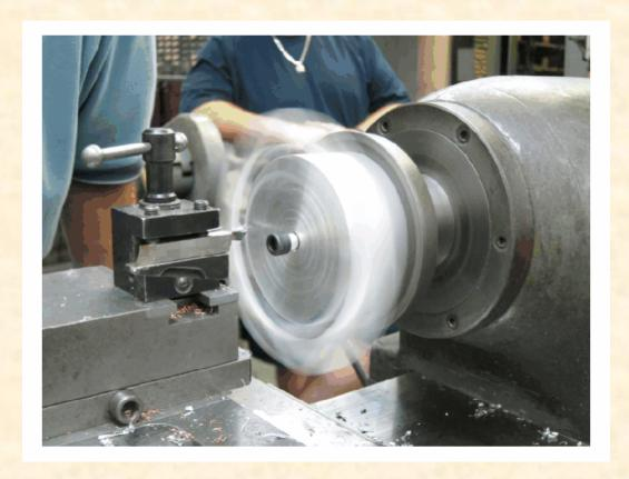
Allesandro cut the channels in the plates to allow for the insertion of a gasket to provide a watertight seal.
