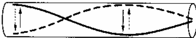
Standing wave pattern at second harmonic frequency ( f_2 )
