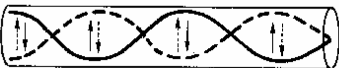
Standing wave pattern at fourth harmonic frequency ( f_4 )
