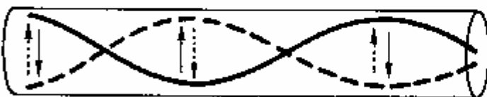
Standing wave pattern at third harmonic frequency ( f_3 )
