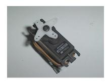
**12 volts DC motor with reduction gearing** – Provides the work to raise or lower the incline. The motor is geared down to increase torque and decrease angular velocity
