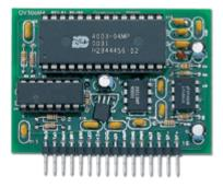
**1 ADC Converter** The Analog to Digital Converter converts an analog potential to a digital signal which can be interpreted by the Basic Stamp
