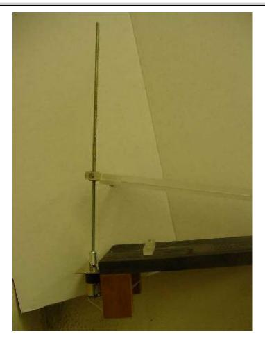
As the cart comes down it interrupts two photogates which consists of an Infrared Emitter Diode and a Phototransistor. The the cart travels along the track and interrupts the photogates, sending a signal to the Basic Stamp
