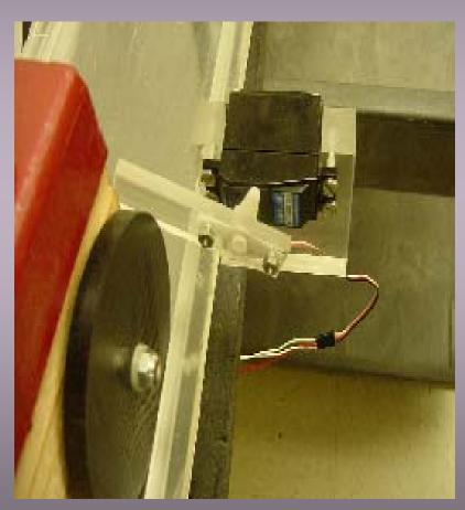
Once the incline reaches the proper angle a signal is sent to the servomotor instructing it to rotate 90 degrees to release the cart.
