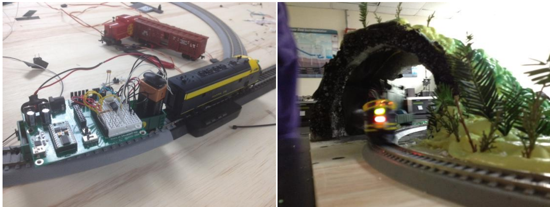
Figure 4: BS2 carrying a light system(left), and train operating under dark conditions; lights on(right)
