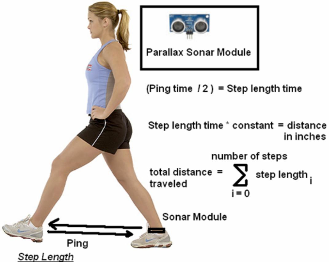
The above diagram explains that as the user takes a step, the sonar module is triggered and measures the distance between the back of the heel of the user and the sonar module. This distance is equivalent to the step length and can be used to determine how far the user traveled in a particular compass direction.
