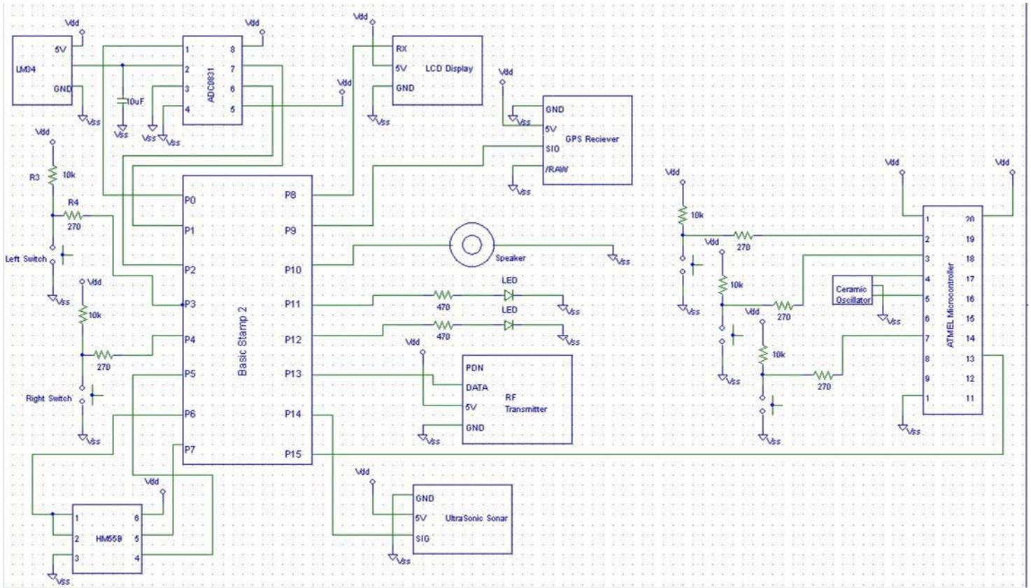
The above diagram shows the electronic circuit diagram for the Future Soldier System. In a production model, the system would include more IO pins and use printed circuit board and surface mount technology to reduce size and cost.
