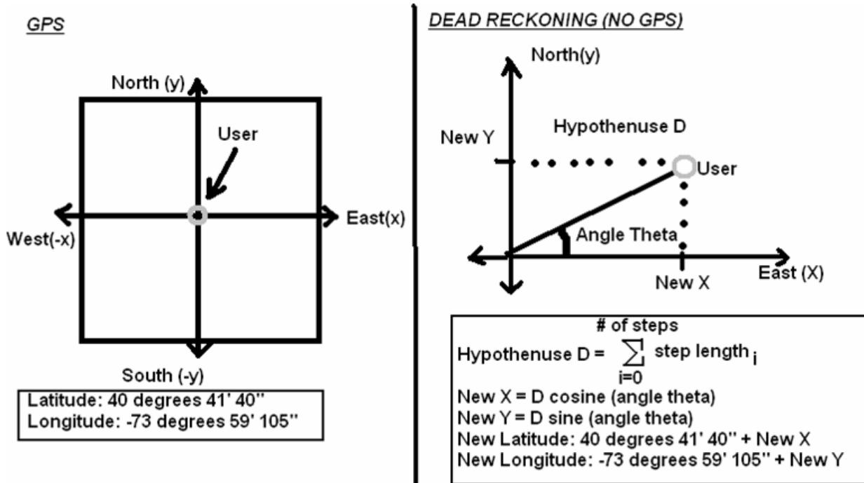
In the GPS environment, the user's current positioning data is updated and broadcast over RF every second. In a non GPS environment, the microprocessor reverts to the dead reckoning module. As illustrated in the above diagram, as the user moves in the first Cartesian quadrant, the user's new latitude and longitude can be calculated as the sum of the last known and good GPS coordinate with the X and Y offset from the dead reckoning module.
