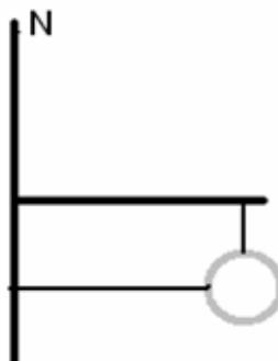
As the user moves around in a non GPS environment, the dead reckoning module uses a series of continuous approximations to calculate the user's latest position. The microcontroller has access to two key mathematical numbers; the first is the step length of the user and the second is the angle theta that the step was taken in relative to magnetic
